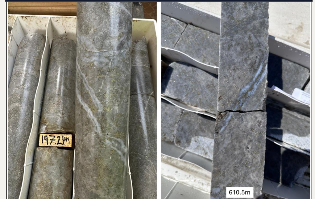
Core Photos of Quartz-Sulfide “B-Type” Veins in Hole 37
