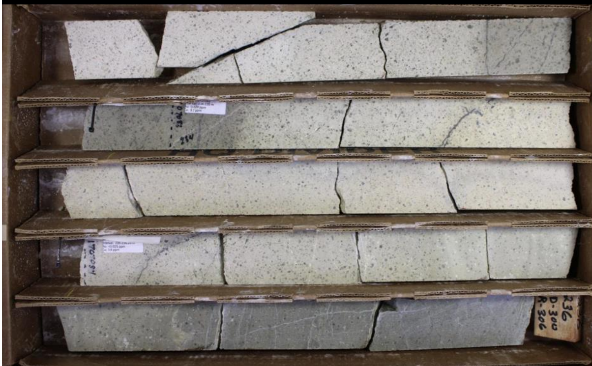
B20C-007 @ 236 m: quartz-feldspar porphyry dyke with thin sphalerite-galena veins
