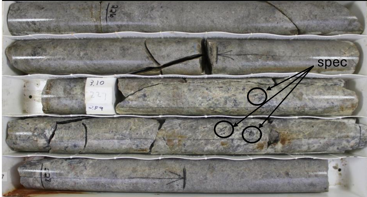
B24C-024 @ 227 m: quartz-alunite+white mica alteration with local specularite (spec)
