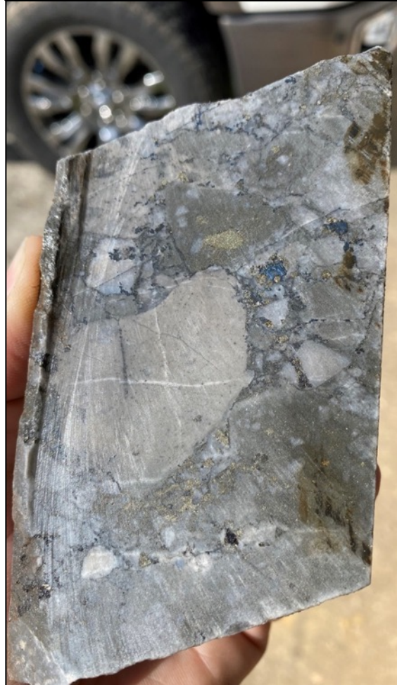
Sub-rounded, polyphase, clast-supported, sulfide clasts and matrix: note covellite in center
