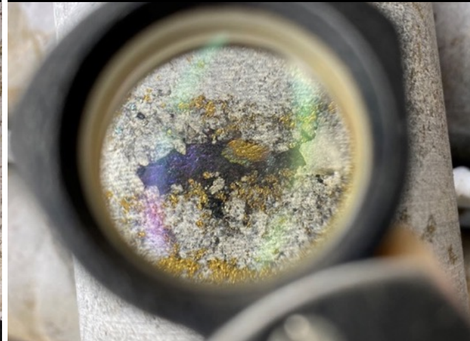
B21C-16: 223m. Chalcopyrite + Bornite
