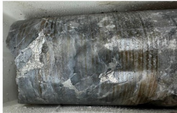
Quartz-telluride vein at 171m
