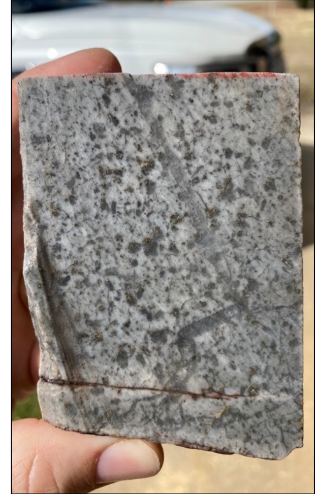
Large, mineralized quartz-porphyry clast within breccia
