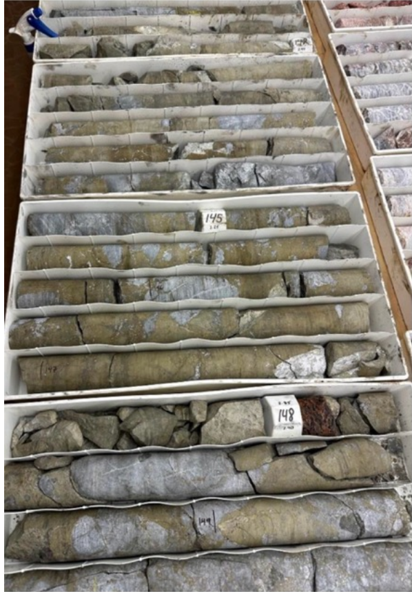
Massive sulfide interval from ~140-149m
