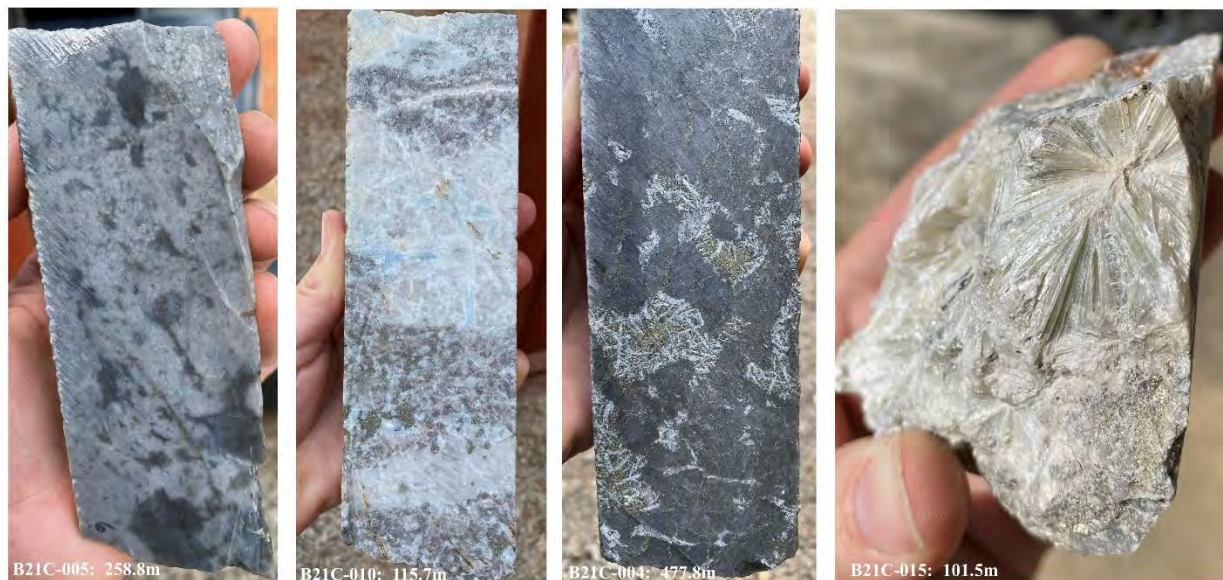
Figure 7-6: Examples of quartz-aluminosilicate rocks (Alx). Left: patchy quartz-topaz alteration; left center: coarse kyanite “skarn”; center: “gusano” texture defined by patchy kyanite+pyrite; right: coarse, radiating pyrophyllite
