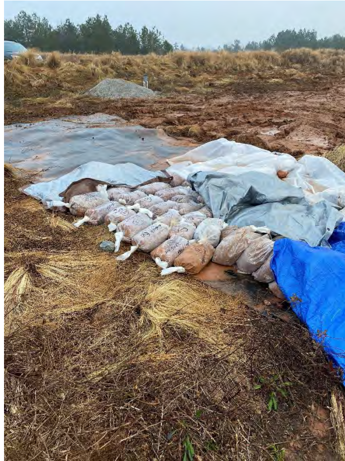
Figure 11-3: Sonic Samples Collected at the Rig. Photo December 13, 2020
