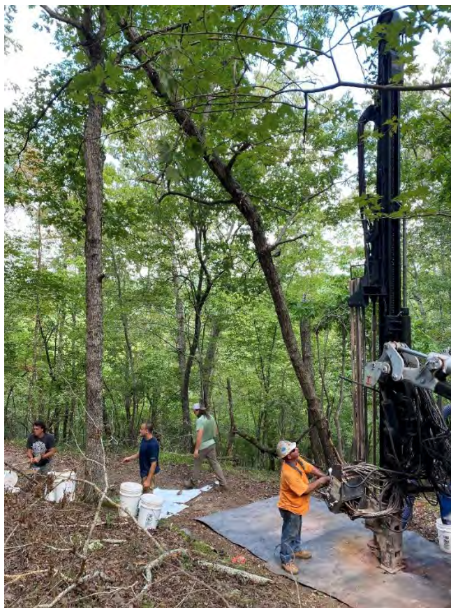
Figure 11-2: Typical RAB set up. Photo August 28, 2020
