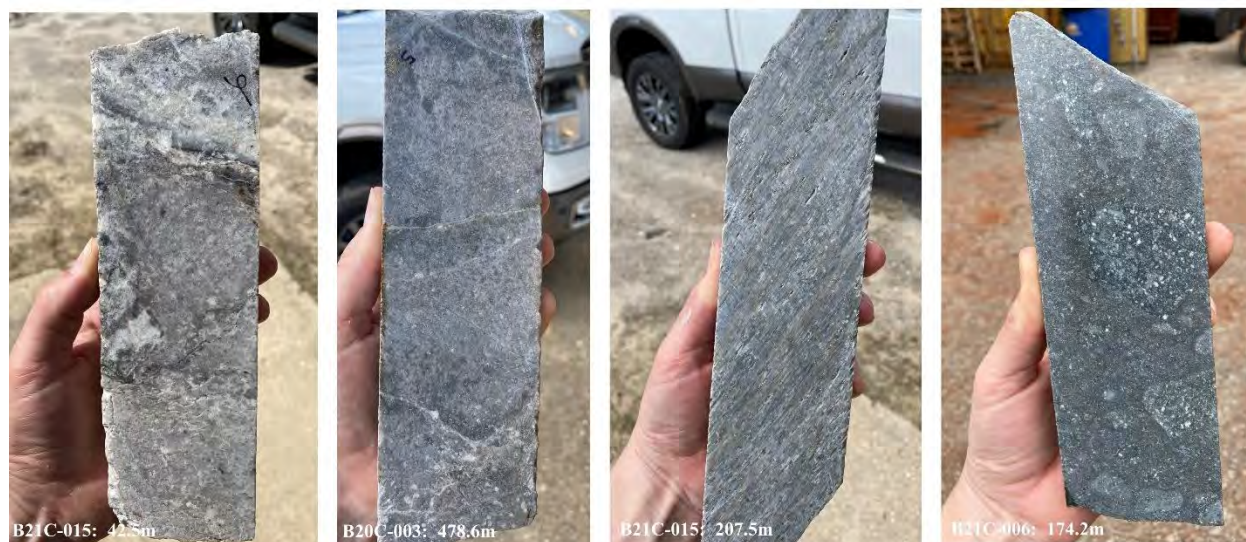
Figure 7-5: Progression of Brewer alteration styles and intensities decreasing from left to right
