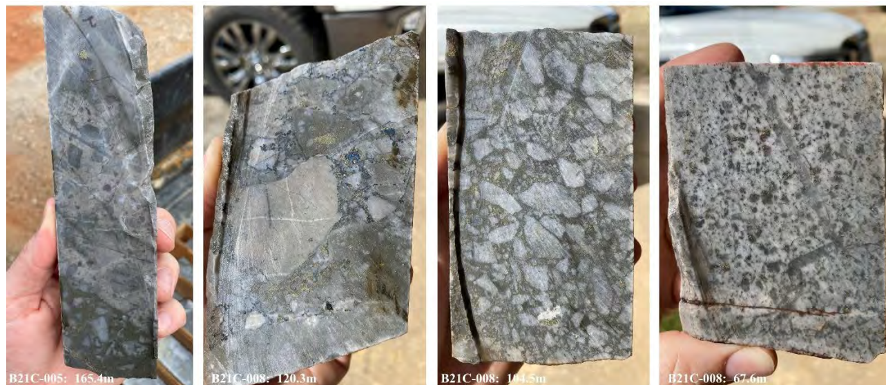
Figure 7-7: Examples of breccia types recognized at Brewer. Left: brecciated clasts indicate multiple phases of brecciation; Left center: sub-rounded clast supported breccia; Right center: monolithic, angular, clast supported breccia; Right: large quartz-porphyry clast with deformed quartz vein
