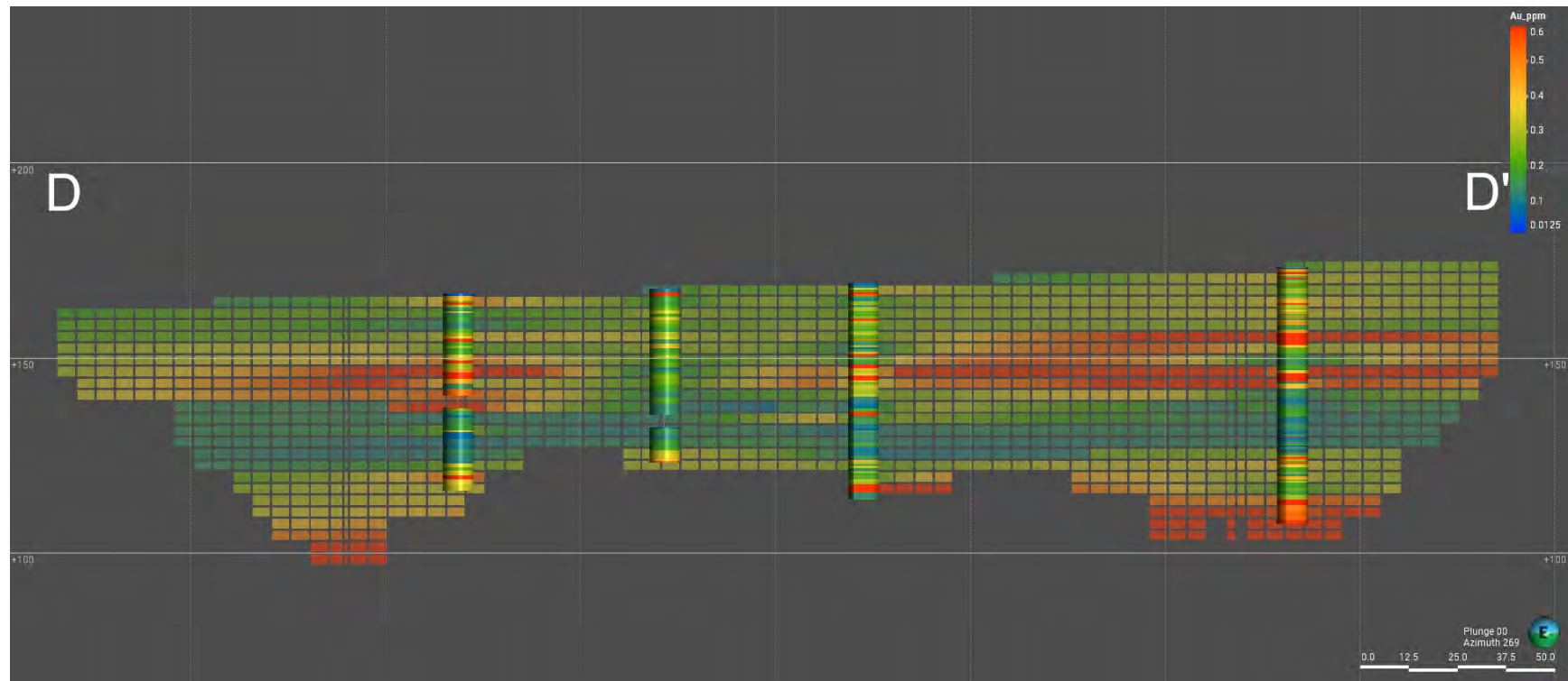
Figure 14-43: Section D-D' Showing Au Backfill Blocks and Associated Sonic Drillholes, All Estimated Backfill Domains, Looking West
