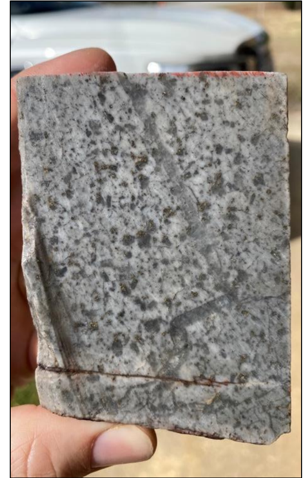
Large, mineralized quartz-porphyry clast within breccia
