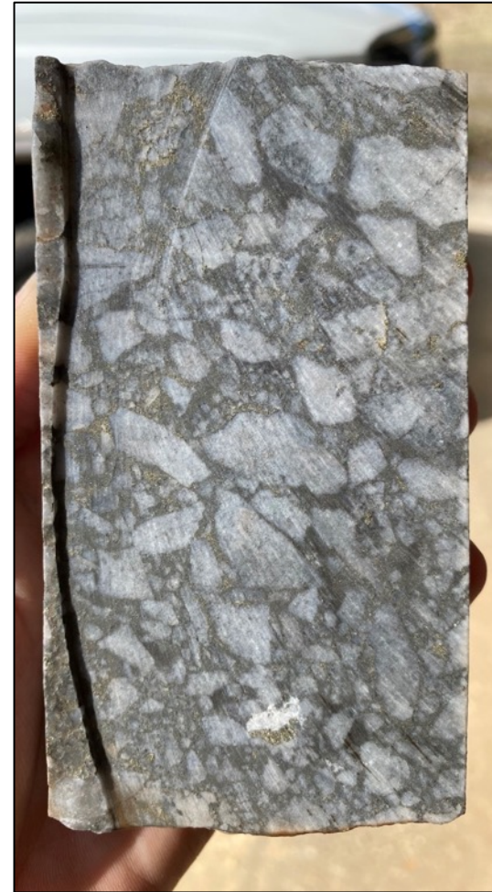
Angular, monolithic, matrix-supported
