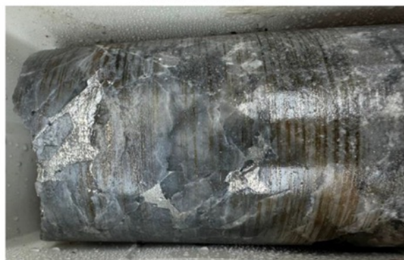
Quartz-telluride vein at 171m
