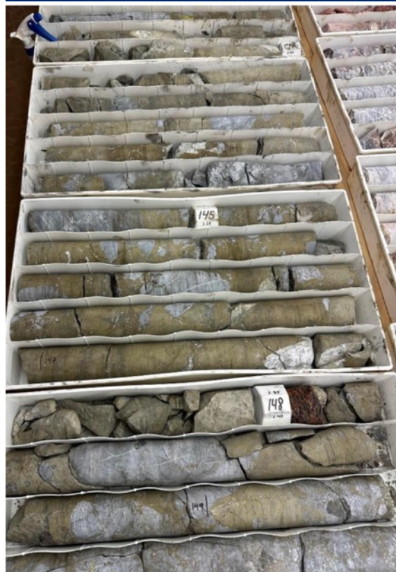
Massive sulfide interval from ~140-149m
