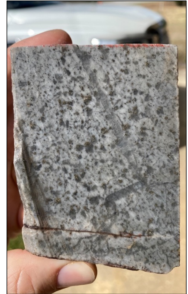
Large, mineralized quartz-porphyry clast within breccia
