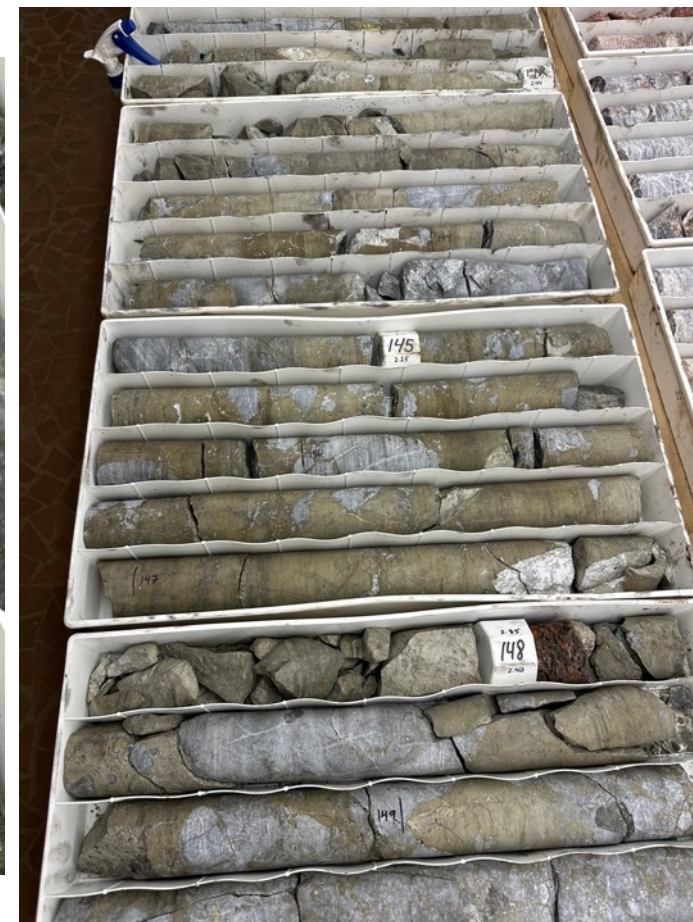
Massive sulfide interval from ~140 – 149 m
