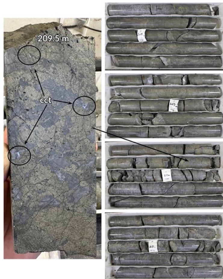
Massive sulfide zone from 203 to 213 m depth. Note chalcocite (cct), a copper sulphide mineral at 209.5 m
