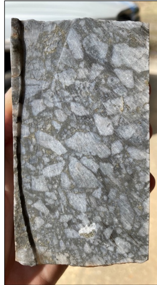
Angular, monolithic, matrix-supported
