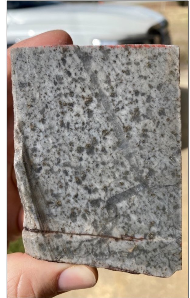
Large, mineralized quartz-porphyry clast within breccia
