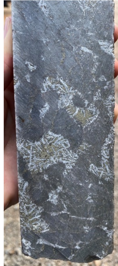
SWIR: K-P-T + alunite. Patchy "gusano" texture defined by kyanite + py
